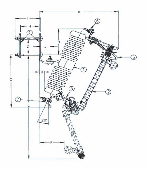
Fig. 1. Typical arrangement of 11 kV Fuse Cutout.
